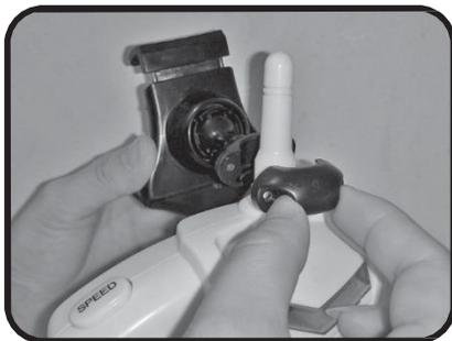
3. Install the bracket around the antenna of the radio.
